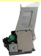
The SHT series can feed and dispense regular cards as well as those with special form factors such as sleeved cards and cards which do not conform to the ISO / IEC 7810 standards.
